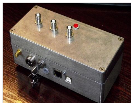
Fig. 1. The data acquisition system in the implementation of a three-channel.
