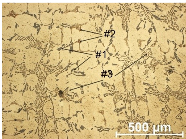
Fig. 6. \text{AlSi6Cu4} alloy after solution in 475^\circ\text{C}
