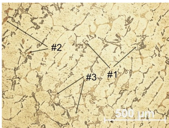
Fig. 9. \text{AlSi8Cu3} alloy after solution in 475^\circ\text{C}
