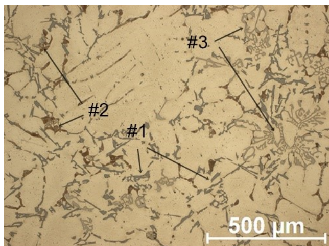
Fig. 5. \text{AlSi6Cu4} alloy after thermal-derivate analysis. #1 - \beta phase, #2 - \text{Al}_2\text{Cu} , #3 - \text{Al}_{15}(\text{Fe}_3\text{Mn})_2 phase
