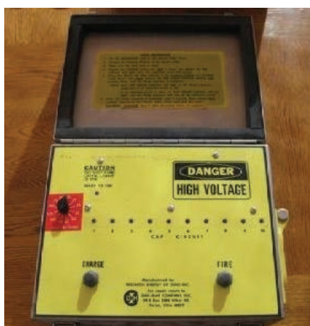
Fig. 7. Sequential blasting machine REO BM 125-10b ( https://www.worthpoint.com/worthopedia/sequential-blasting-machine-bm125-10b ) Rys. 7 Zapalarka sekwencyjna REO BM 125-10b ( https://www.worthpoint.com/worthopedia/sequential-blasting-machine-bm125-10b )
