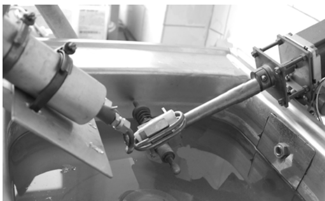
Fig. 2. The inductor (left) and the specimen holder (right)
