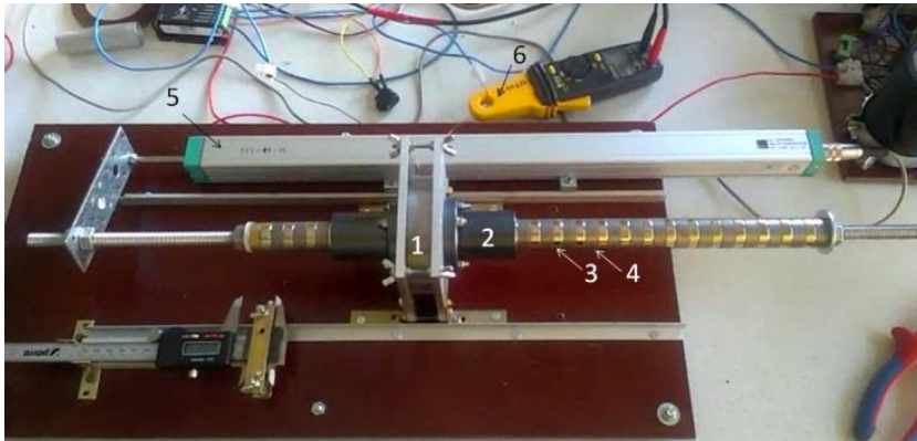
Fig. 9. The laboratory linear actuator permanent magnet tubular linear actuator: 1 — coils with ferromagnetic case, 2 — linear bearing, 3 — permanent magnet ring, 4 — ferromagnetic ring, 5 — position sensor, 6 — specialize current sensor 'center 223'
