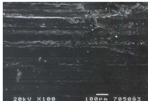
Fig. 7. Photomicrograph of sliding surface of the AlMg10 + (7% SiC and 3% C gr ) composite, magn. 100×
