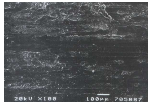
Fig. 6. Photomicrograph of sliding surface of the AlMg10 + (5% SiC and 5% C gr ) composite, magn. 100×
