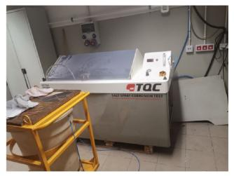
Figure 1 Photograph of the salt spray chamber in SaMASZ. Source: own study
