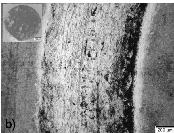
Fig. 7. Worn surfaces of G3 specimen against its 100Cr6 (a) or its alumina counterpart (b) shown at upper left corner
