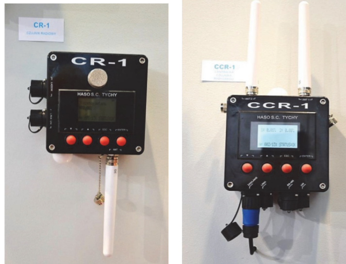
Fig. 1. Devices of the new gas measuring system [11]
