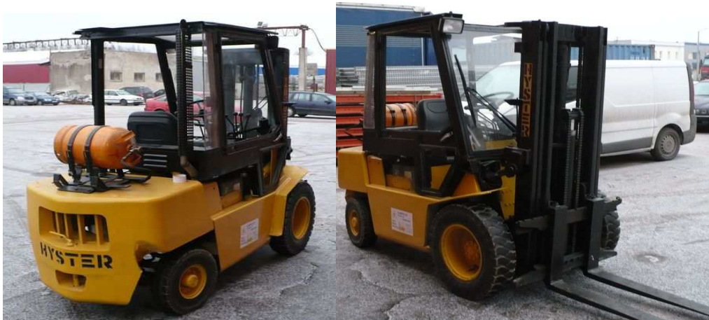
Fig. 5. The counterbalanced forklift truck discussed in case study
