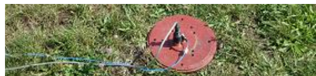
Fig. 5. Attaching the vibration sensors
