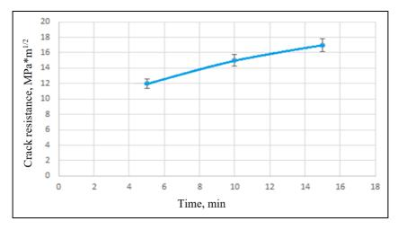
Fig. 3. Dependence of crack resistance of a covering on time of spraying (own study)
