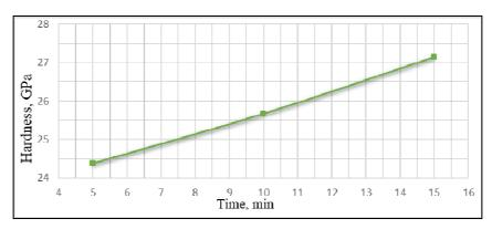
Fig. 2. Dependence of hardness of a covering on spraying time (own study)
