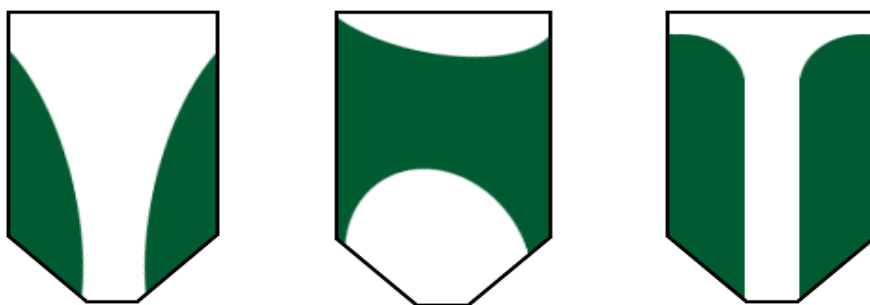
Fig. 2. Problematic phenomena in silos: funnel, arch, centric tunnel (from the left to the right)
