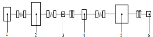
Fig. 1. Experimental setup: 1 – electric motor; 2 – flywheel; 3 – torque meter; 4 – MR damper; 5 – electromechanical transducer; 6 – encoder
