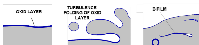
Fig. 1. Scheme of the bifilm creation process
