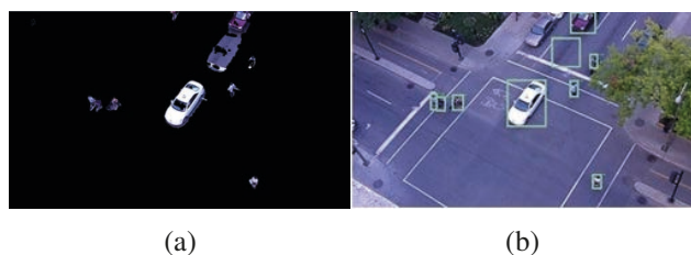
Figure 9. Example result of performing AND operation between ViBe result and the original image before inputting to the neural network for object detection.
