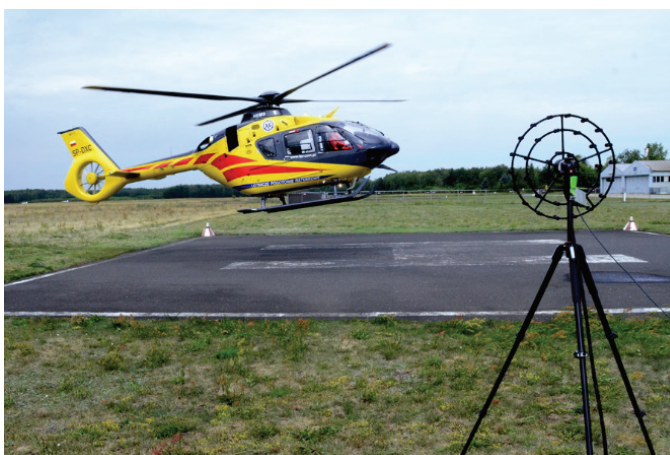
Fig. 4. Testing the noise sources of the landing helicopter and a directional diagram of the amount of noise emitted by the helicopter at the helipad
