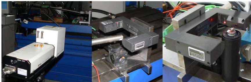
Fig. 7. Comparing the Blum Novotest LaserControl to a laser vibrometer
