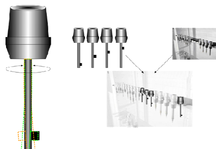
Fig. 10. Adjustable exciter for specific load of main spindle
