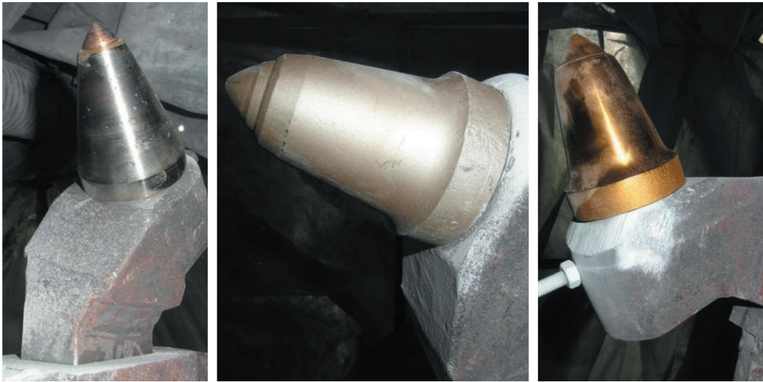
Fig. 7. Examples of tangential-rotary picks prepared for testing
