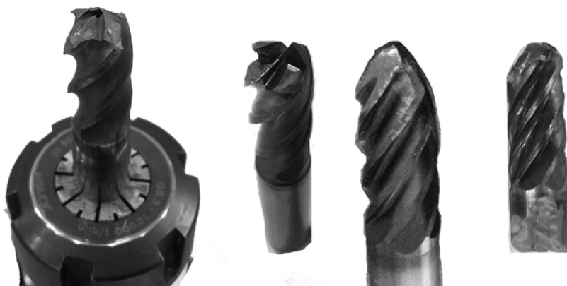
Fig. 3. Examples of cutters subject to failure
