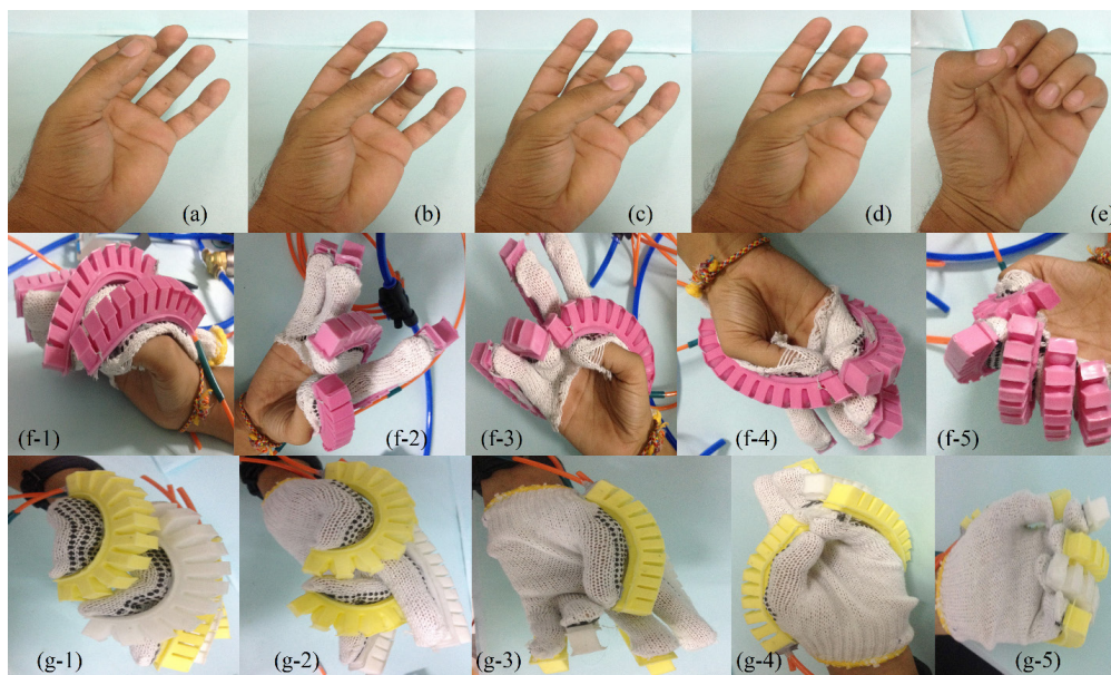
Fig. 11. Kapandji test for rehabilitation purpose: (a) thumb contact with index finger (b) thumb contact with middle finger (c) thumb contact with ring finger (d) thumb contact with small finger (e) full hand flexion (f-1 – f-4) soft robotic glove assembled with RTV 225 performing all above posture (g-1 – g-4) robotic glove performing the human hand posture for rehabilitation standardized test.
