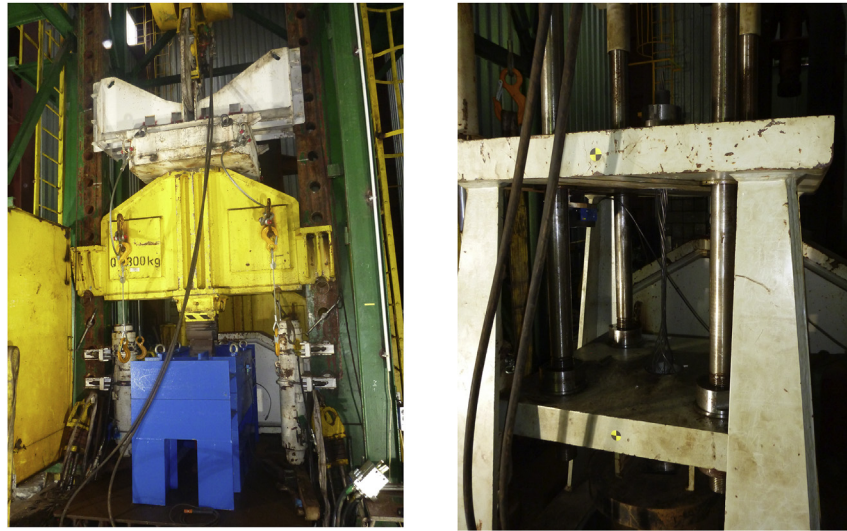
Fig. 2 – View of testing stand with construction elements for impact tests of transverse and longitudinal loads of steel wire ropes.
