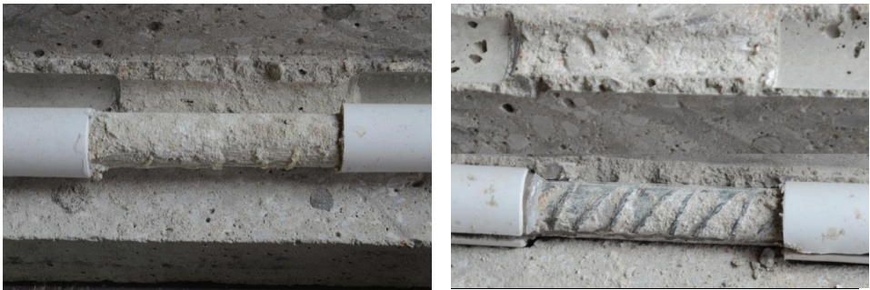
Fig. 5. Failure of the GFRP bar (GS-18-5.3) and steel bar (S-16-5.3) along the embedded length
