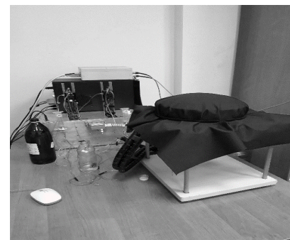
Fig. 2. Setup for measurement and evaluation of thermodynamic parameters in a system simulating a real human body - material/textile system
