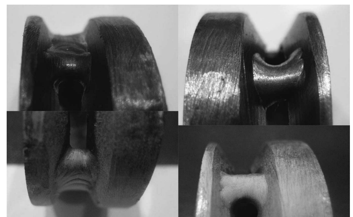
Fig. 13. Elimination of cracks by applying pre-heating to temperature of 150^\circ\text{C}
