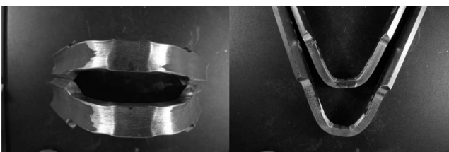
Fig. 7. Results of bend test – root side
