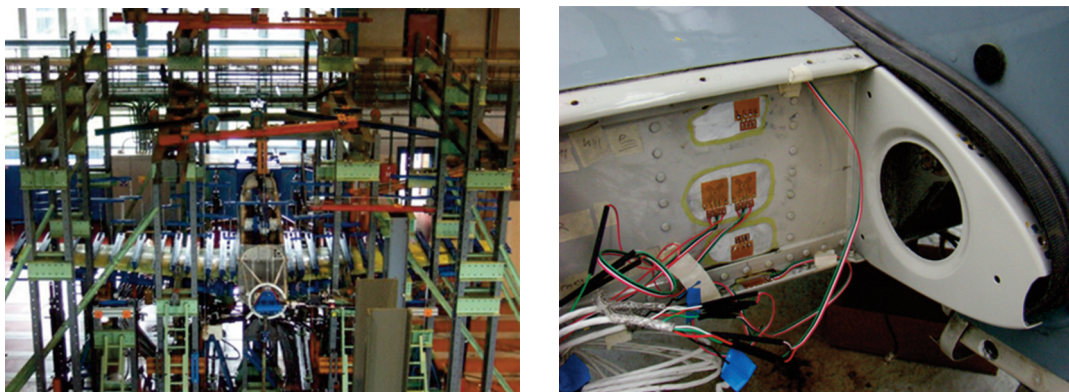
Figure 1. Test specimen mounted in the test rig and the right front wing spar with installed strain gages.
