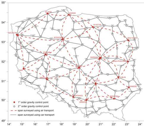
Figure 1. First gravity control network in Poland
