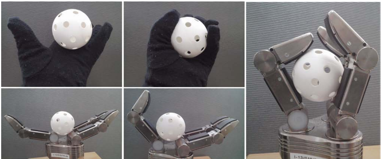
Fig. 6. Calibration of the spherical grip (from left): hand and gripper open, hand and gripper at the beginning of the calibration process (large discrepancies in the pose of two fingers), spherical grip after calibration
