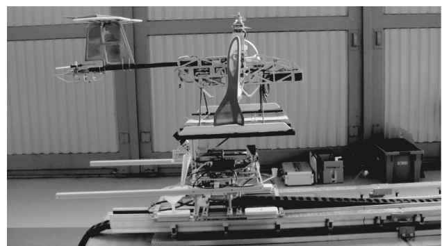
Fig. 2 . Prototype UAV catapult based on Meissner effect
