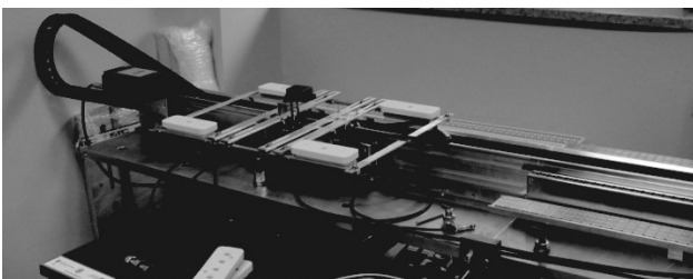
Fig. 3. Prototype catapult based on Meissner effect, built as part of 7 PR UE GABRIEL
