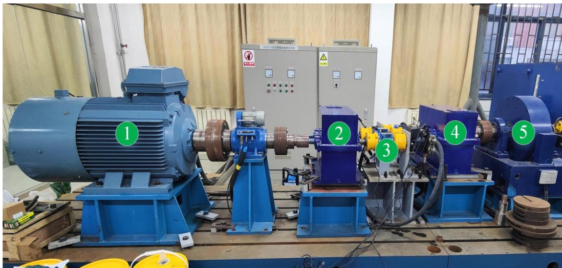
Fig. 21. Picture of the experimental setup (1) motor, (2) transfer gearbox, (3) speed-torque sensor, (4) differential gearbox, and (5) dynamometer.
