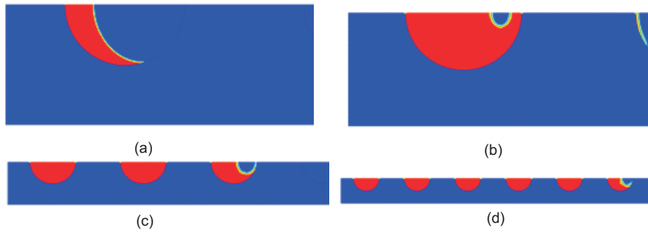
Figure 10: The melted fibre material for the case of the nonisothermal phase change and different degree of dispersion (a) 8 fibres (after t = 365 s), (b) 16 fibres (after t = 401 s), (c) 32 fibres (after t = 726 s), (d) 64 fibers (after t = 743 s).
