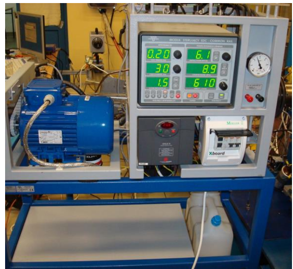
Fig. 6. Test stand for high-pressure pump and injectors in Common Rail fuel injection system
