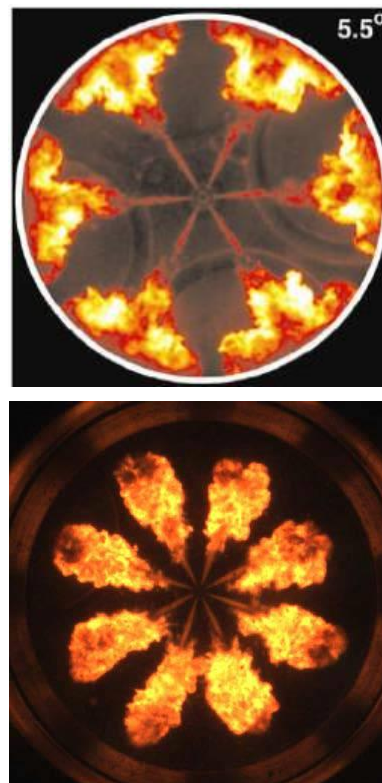
Fig. 1. Propagation of flame in conventional self-ignition engine with direct fuel injection [8]
