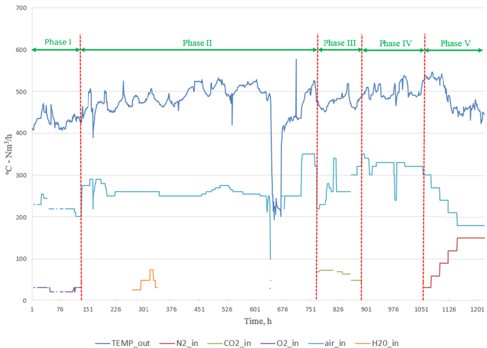
Fig. 2. Temperature of the syngas and amounts of gasifying agents in Nm 3 /h used during the UCG process during the different phases of the experiment
