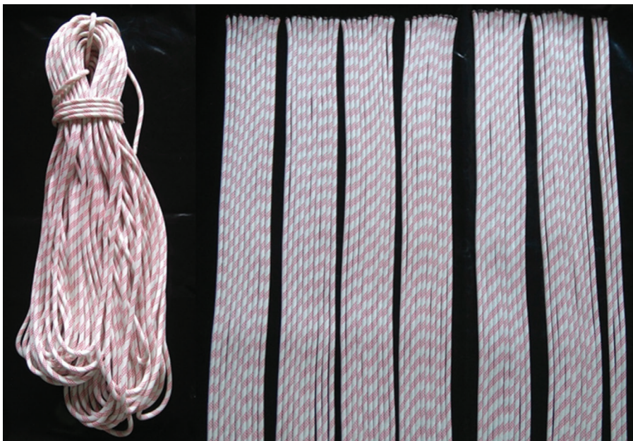
Fig. 3. Edelweiss BUD rope before and after dividing into sections
