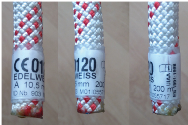
Fig. 2. Marking of the tested rope
