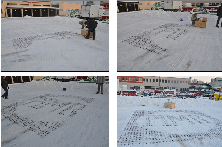
Fig. 6. Field test: a) original image; b) converted image; c) seeding the logo of the Industrial Institute of Agricultural Engineering (PIMR) on the snow
