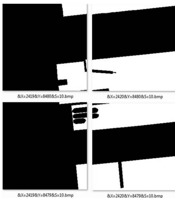
Fig. 2. Monochromatic map pictures with their names chosen from hierarchical layer of tile map pyramid, conforming to S = 10 scale
