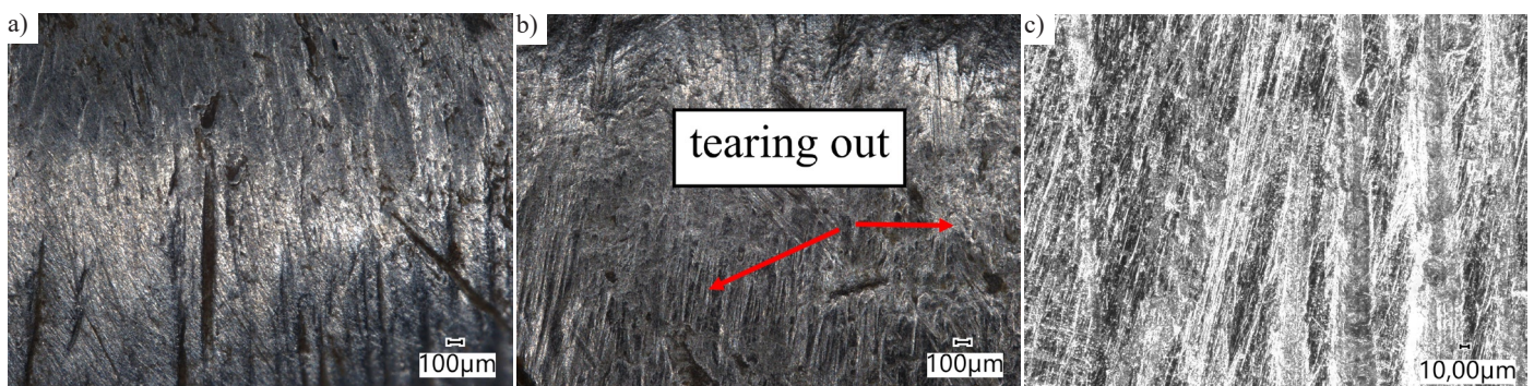
Fig. 11. The appearance of the specimen surface after being worn in a heavy soil: (a) 38GSA steel; (b) ELHARD70; (c) chisel
