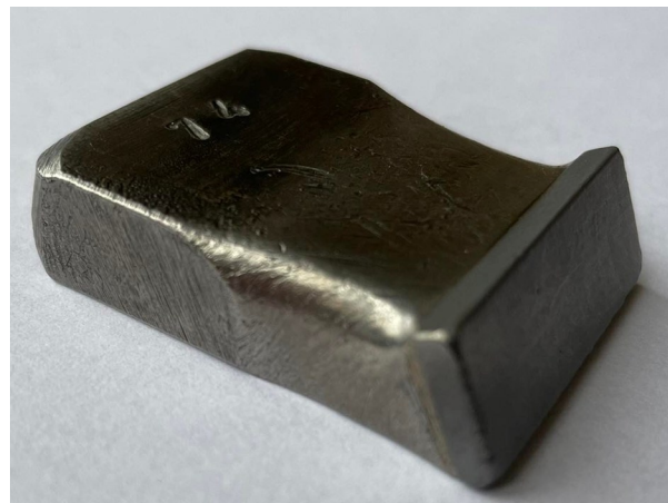
Fig. 13. The division of volumes for the specimen with sintered carbide G10: (a) 3D scan; (b) the actual specimen with sintered carbide G10
