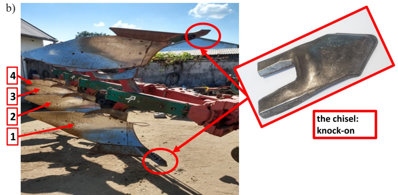
Fig. 7. Method of mounting: (a) a specimen in the holder; (b) a chisel
