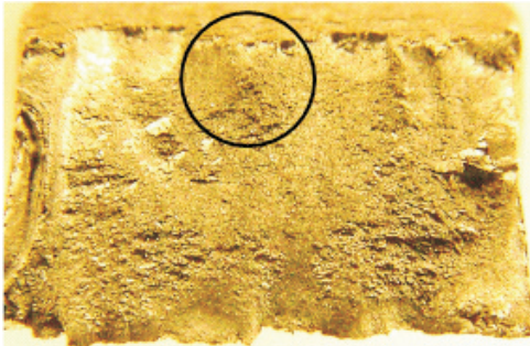
Fig. 4. View of the macrostructure of fatigue crack S960QL steel samples
