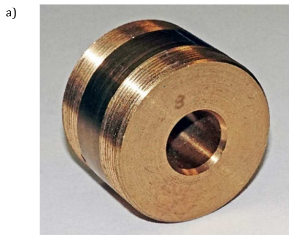
Fig. 13 Calibration nozzle in accordance with EN 250:2014 : (a) nozzle design, (b) method of mounting the nozzle on the test bench.
