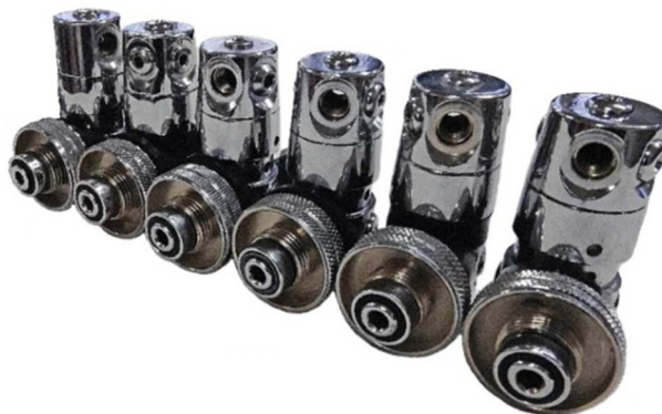
Fig. 3 Randomly selected first stage reduction units selected for testing the breathing apparatus.
