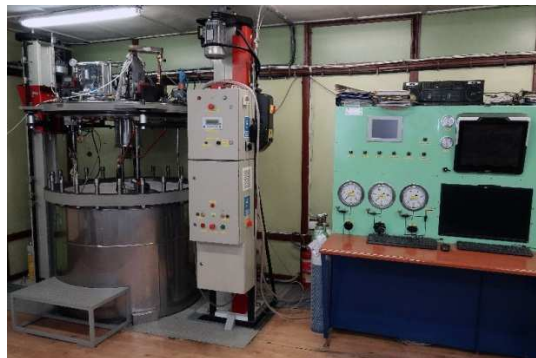
Fig. 12 Test bench – a breathing simulator.
