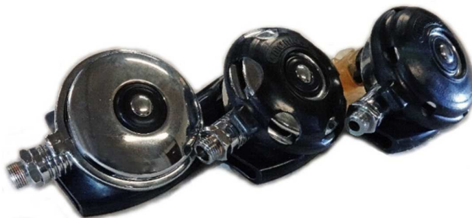
Fig. 7 Randomly selected second-stage units of a selected breathing apparatus.
