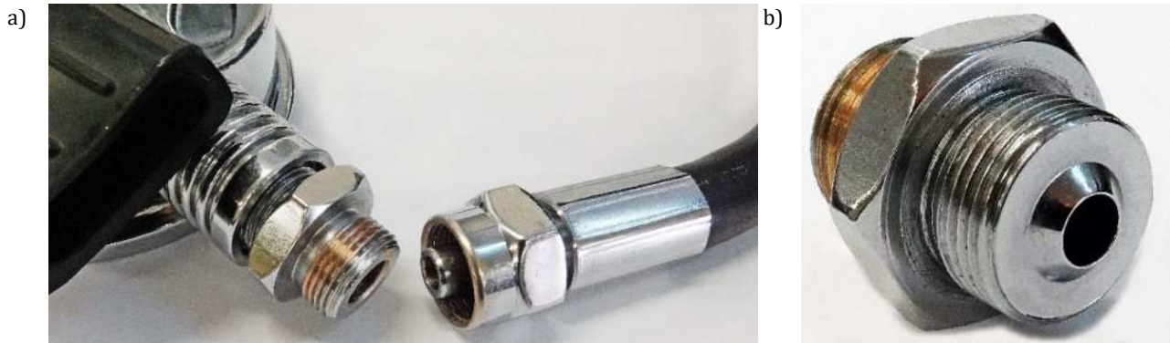
Fig. 10 Nozzle of the concurrent pressure reducing valve of the breathing apparatus : (a) location of the nozzle in the second stage throttling valve from the housing side; (b) appearance of the original nozzle from the contact side of the movable plug cutting off the flow of breathing gas.
