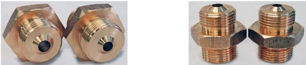
Fig. 11 View of additionally fabricated nozzles for the concurrent pressure relief valve of the second stage of the breathing apparatus.
