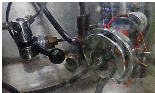
Fig. 16 Method of inserting a breathing apparatus into a breathing simulator.
