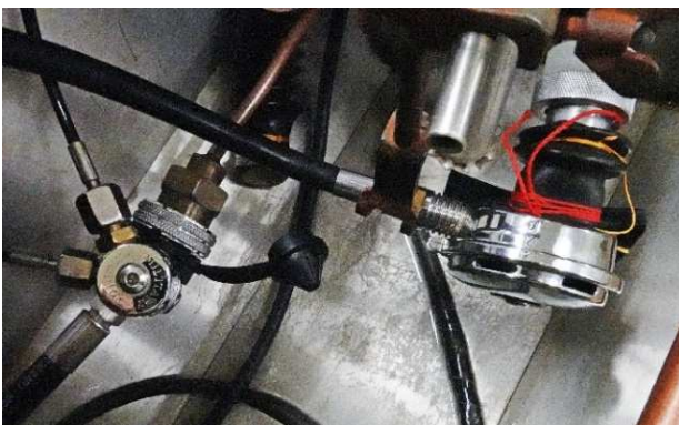
Fig. 16 Method of inserting a breathing apparatus into a breathing simulator.
