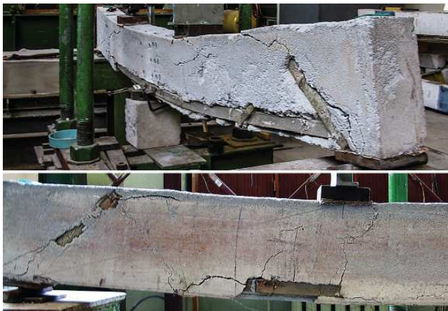
Fig. 3. Process of the experimental samples destruction of type B-1 (see above) and type B 5 (see below)
