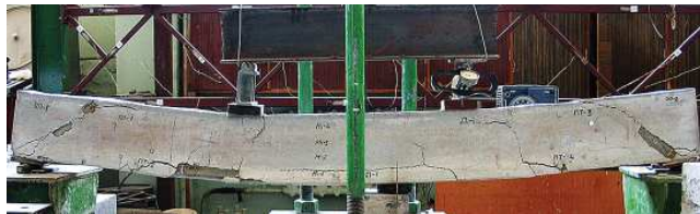
Fig. 4. General view of the experimental sample of type B-5 after destroying
