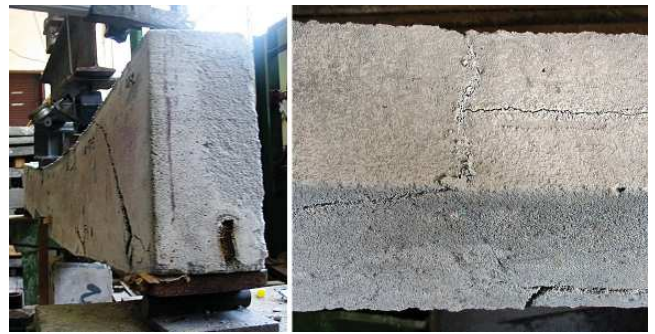
Fig. 5. Destruction features of the experimental samples: the slip of the bamboo at the end of the beam in type B-2 (see on the left) and the appearance of longitudinal cracks on the upper edges in type B-3 (see on the right)
