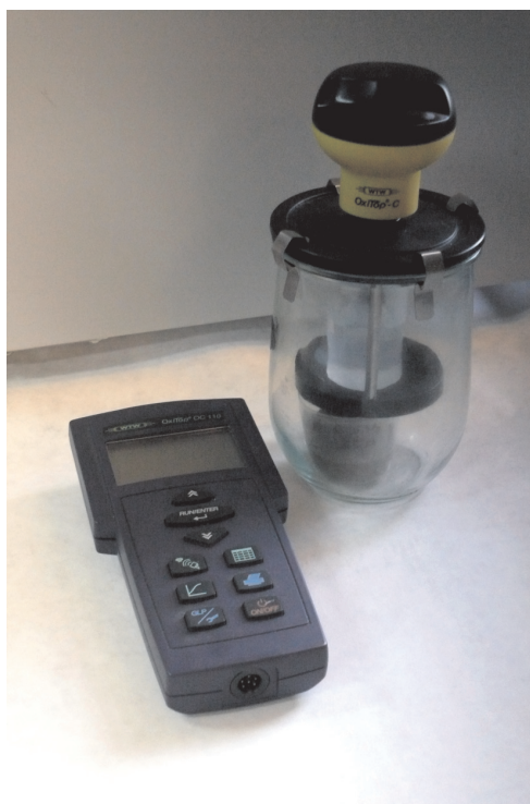
Fig. 2. A photo of equipment for measuring a demand for oxygen (photo: M. Kopec)
