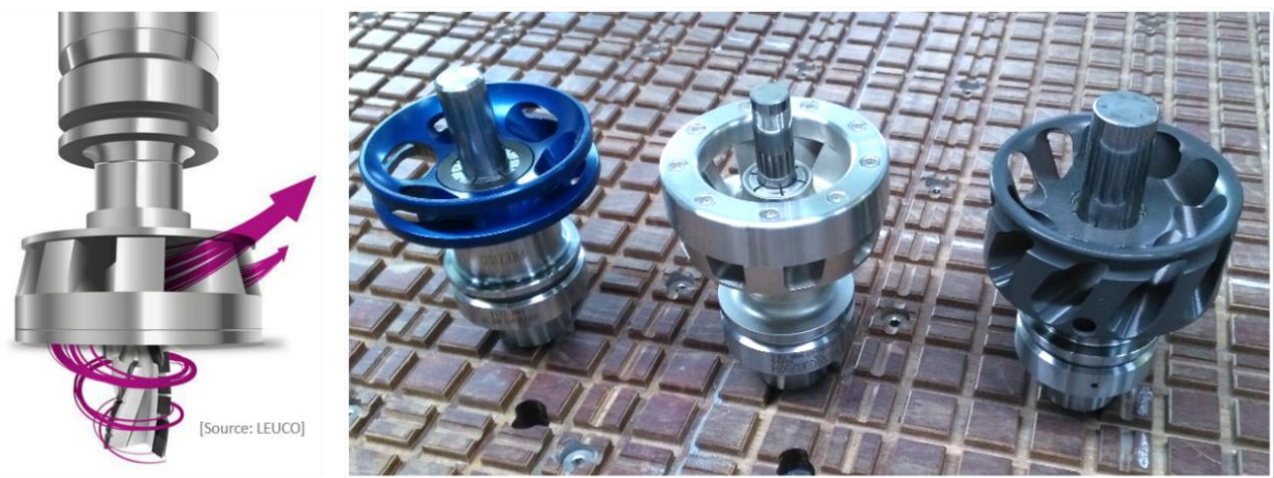
Fig. 12. Turbine shaped chip evacuation systems at wood machining tools [LEUCO, IfW]
