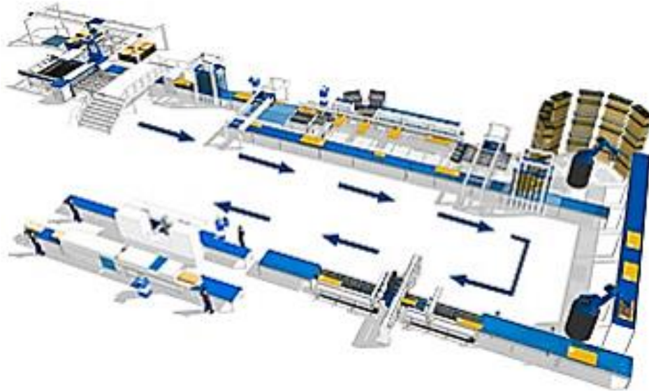
Fig. 5. Automated wood processing production line [source: HOMAG]
