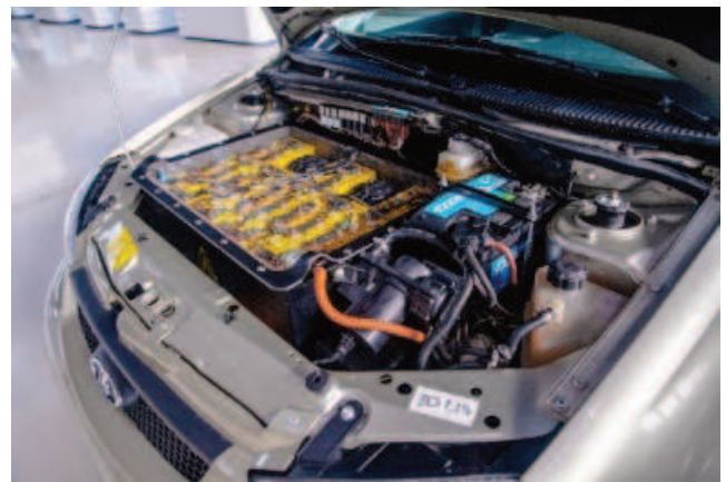
Fig. 5. General view of the engine compartment with the developed system of accumulation and storage of electrical energy
