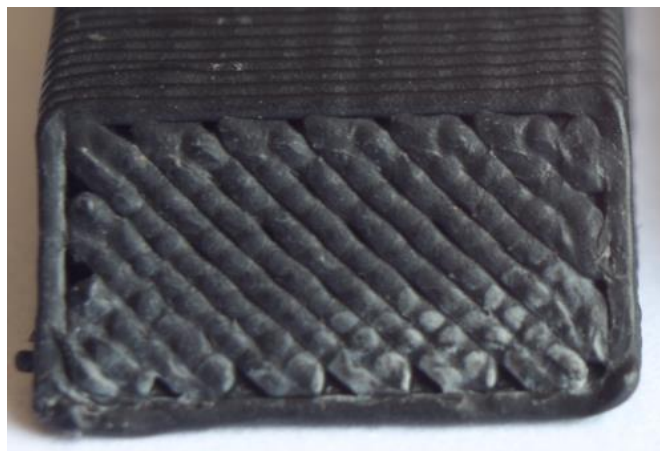
Fig. 1. View of a single layer of a sample manufactured by FDM technology – visible contour and filling threads (thread width approx. 0.5 mm, layer thickness 0.254 mm) [9]
