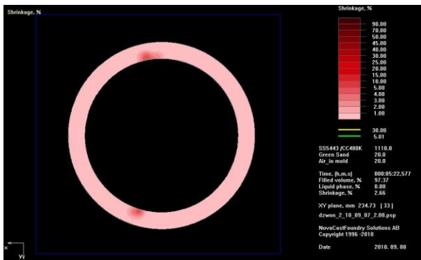
Fig. 13. Shrinkage of a bell casting, transverse cross-section – 3 rd option
