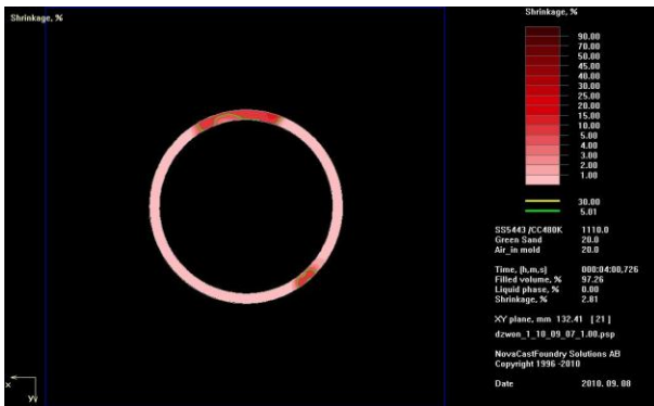
Fig. 7. Shrinkage of a bell casting, transverse cross-section – 1 st option
