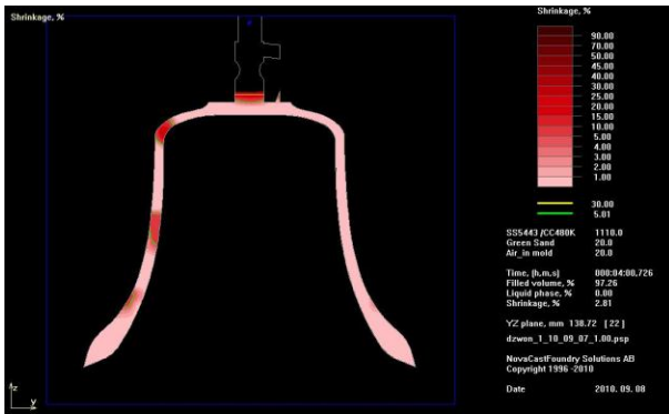
Fig. 6. Shrinkage of a bell casting, longitudinal cross-section – 1 st option
