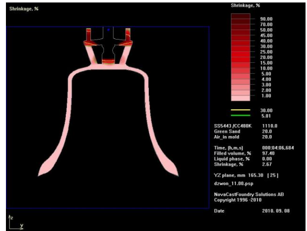
Fig. 9. Shrinkage of a bell casting, longitudinal cross-section – 2 nd option
