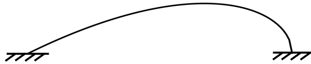
Figure 6. Geometry of Tschirnhausen beam.
