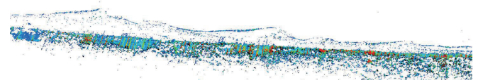
Fig.13. MarLS visualization for the coast fragment with the cloud density parameter of approximately 30 points per m2 for the green colour to approximately 100 points per m2 for the red colour
