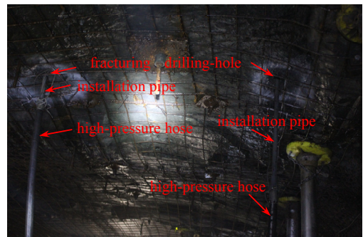
Fig. 10. Hydraulic fracturing in underground coal mine
