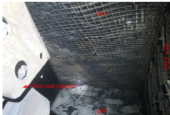
Fig. 4. Hanging roof in the end of longwall mining face
