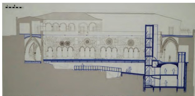
Figure 3. Cathedral of Saint Mary Major in Lisbon. Cathedral cloister; architectural and museum project, cross-section, 2019, photo: M. Barański; designed elements are marked in blue
