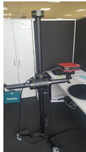
Fig. 10 Scanner 3D GOM ATOS for measurements
