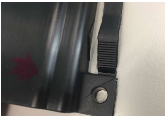
Fig. 5 Burrs and cracks on housing
